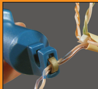
Untwists wire pairs with the innovative wire hook.
