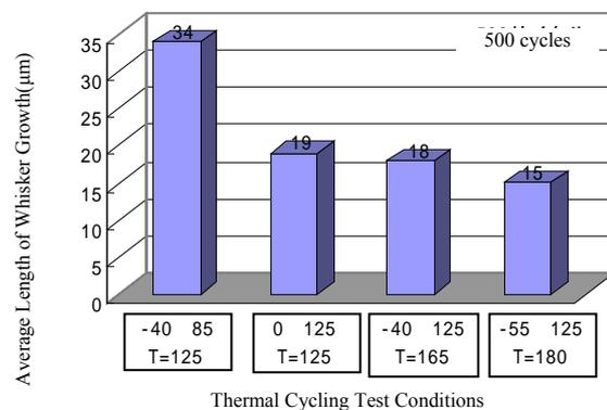
Fig.3 Relation between Temperature difference and Thermal-Cycling Whisker Growth
