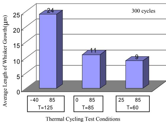
Fig.5 Relation between Low Side Temperature and Thermal-Cycling Whisker Growth
