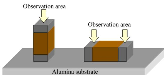
Fig.2 Thermal-Cycling Whisker Observation Area
