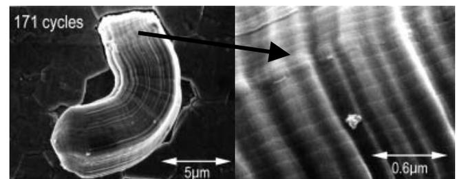
Fig. 13 Magnified SEM Image of Thermal-Cycling Whisker
