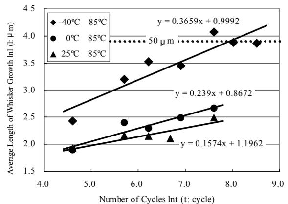
Fig.8 Test Conditions and Thermal-Cycling Whisker Growth
