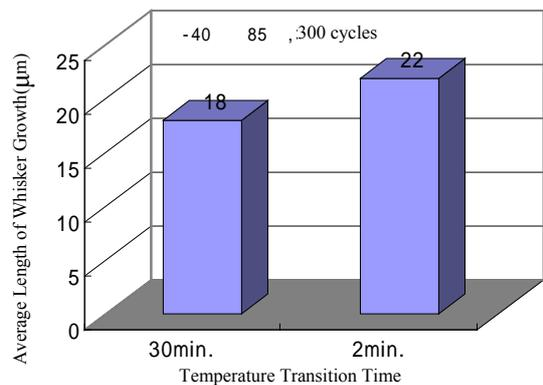
Fig.6 Relation between Temperature Transition Time and Thermal-Cycling Whisker Growth
