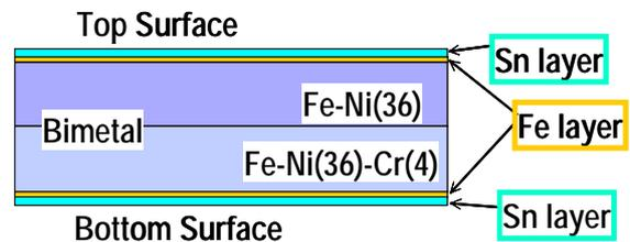
Fig. 16 Bimetal Experiment Substrate
