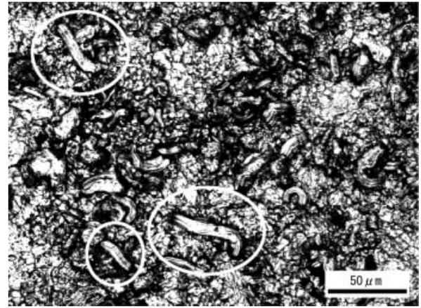
(a) 170 $^{\circ}\text{C}$  Pre-soldering (hot plate method), Average length 32 $\mu\text{m}$
