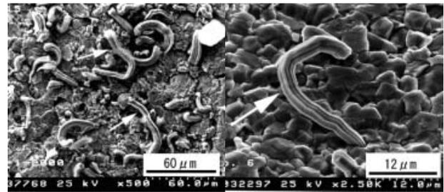
Fig. 1 SEM Image of Thermal-Cycling Whiskers
