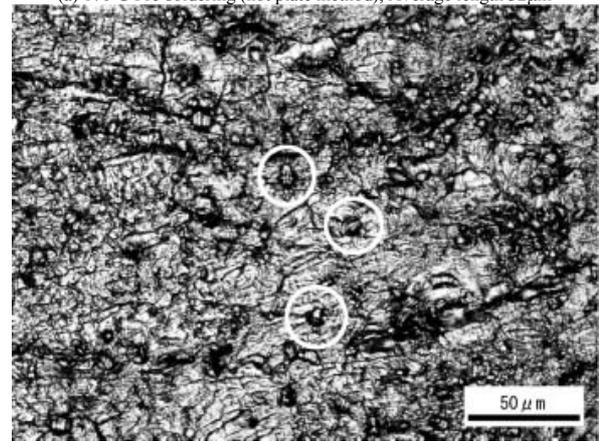
(b) 240 $^{\circ}\text{C}$  pre-soldering (reflow method), Average length 9 $\mu\text{m}$
