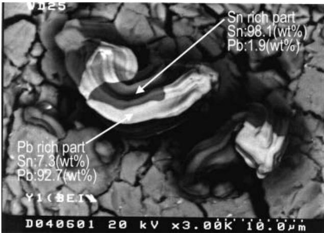
Fig. 15 Reflection Electron Image of Thermal-Cycling Whisker on Solder Plating
