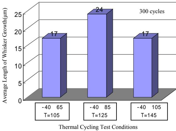
Fig.4 Relation between High Side Temperature and Thermal-Cycling Whisker Growth
