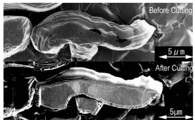
Fig. 14 SIM Images of Cross-Section Surface of Thermal-Cycling Whisker Before and After FIB Processing
