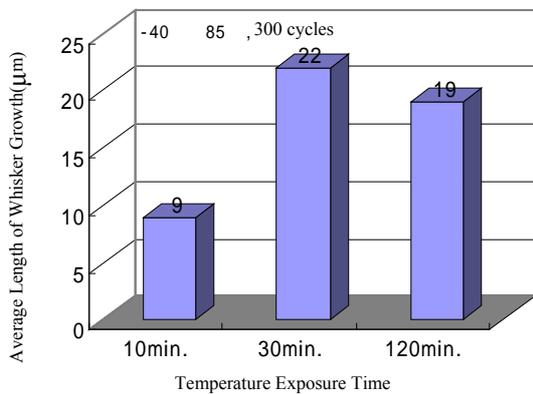
Fig. 7 Relation between Temperature Exposure Time and Thermal-Cycling Whisker Growth
