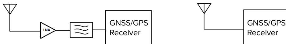
Figure 1: GNSS/GPS single channel receiver (i) single antenna with LNA + pre-filter (ii) single passive antenna
