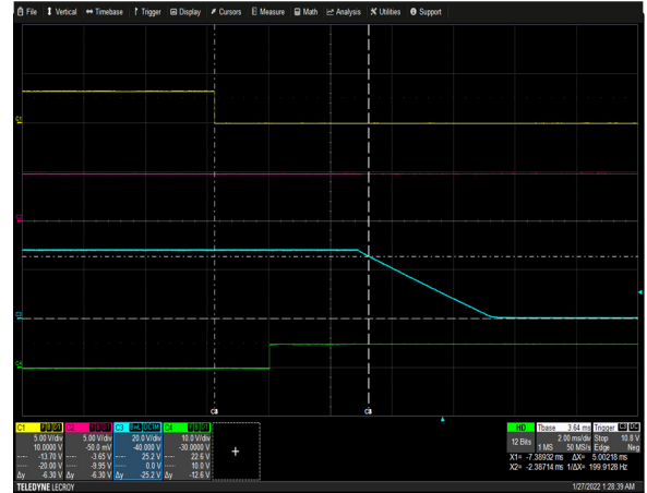
Figure 8: LCC1200-28U-9P Turn Off Characteristic via INH_EN Load: Io = 42.9A (12V), I SB = 1.5A (5V) Ch 1: INH_EN Ch 2: V SB Ch 3: V O CH 4: G_DCOK_C
