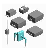
Eaton's high-power transient voltage suppression diodes provide reliable overvoltage protection with very fast response times, low clamping voltage, and high peak current capability.
