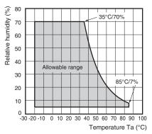
**Note:** No icing or condensation within the operating temperature range.
