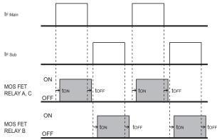
\* Both MOS FET relay A, C and MOS FET relay B may be ON at the same time. For that reason, even if pins 4, 5 and 6 are all connected, please design  $\,$ the circuit so that equipment damage does not occur.
