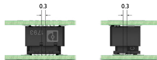
Position tolerance compensation when plugged in
