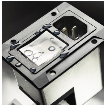
SCHURTER DG12: IEC C14 appliance inlet with mains filter, TA35 circuit breaker, V-Lock cord retention and optional cover for IP67. Available as Medical Version (M80).
