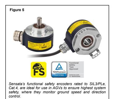
For AGV applications, components that are rated up to Safety Integrity Level 3, or SIL3, are ideal, as this allows for the highest safety level in the system. SIL3-rated encoders can often be more expensive than those of a lower safety rating, but they greatly reduce the risk of failure to the system, which in the case of an AGV navigating a warehouse, could prevent costly damage or injury.
