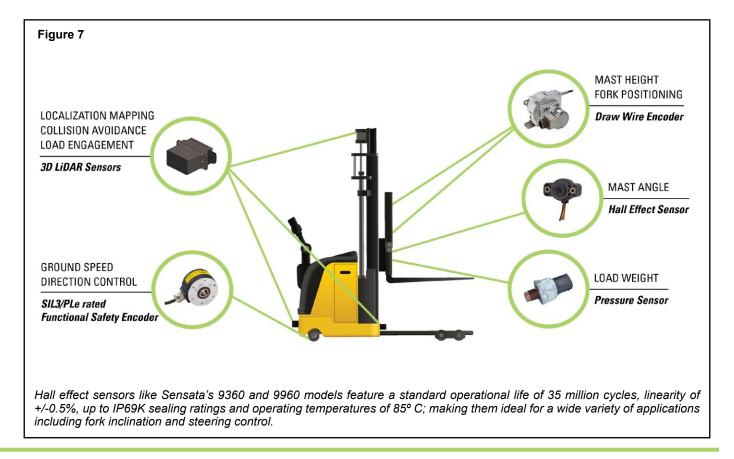
The materials handling sector is one of the most important to designers, manufacturers, and engineers working with sensing and control technologies, and the rise and rise of Automated Guided Vehicles is accelerating the development of new and even more sophisticated sensing solutions.
