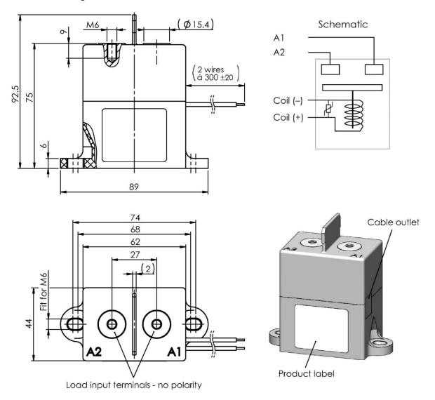
In case of no tolerance shown in dimensional drawing, general tolerances apply: dimension  $\leq 10$  mm;  $\pm 0.3$  mm; dimension 10 to 50 mm;  $\pm 0.6$  mm; dimension > 50 mm;  $\pm 1$  mm
