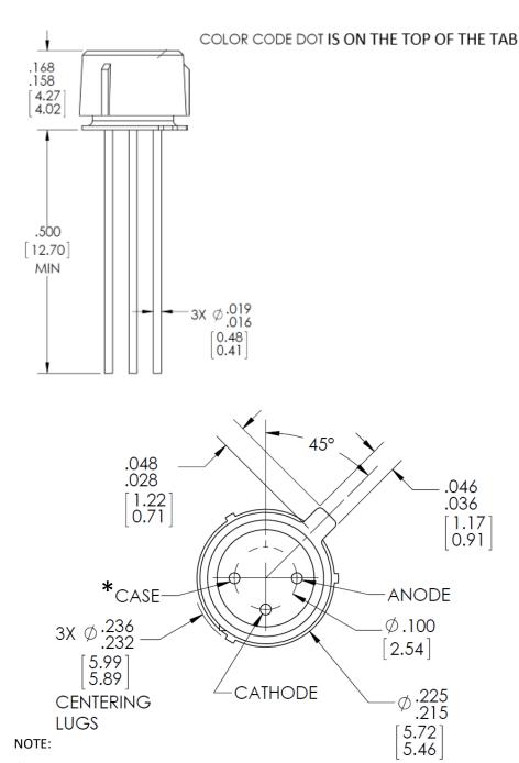
Case is electrically isolated from cathode and anode.
