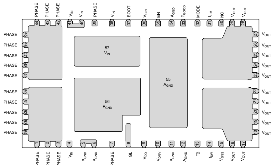
Fig. 4 - Pin Configuration (Top Transparent View)
