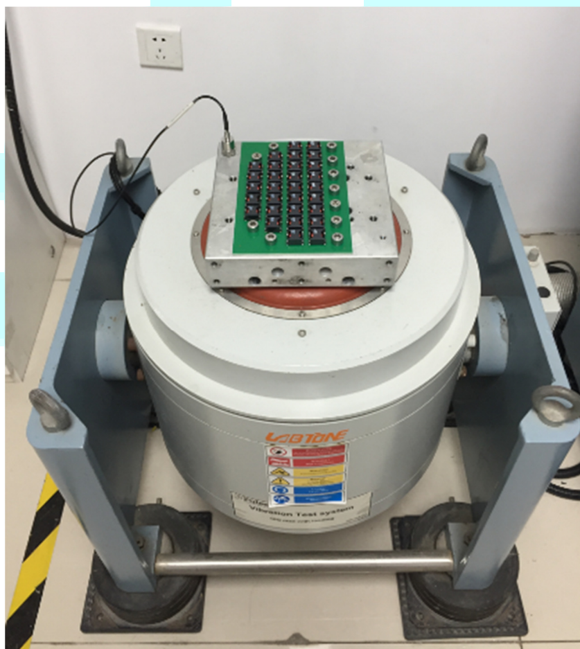
Fig. 2 Vibration Test (X axis)
